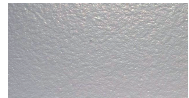
Surfaces prone to wrinkles due to different spraying conditions
